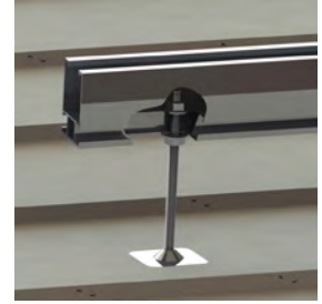
9. Attach rail to the headless threaded bolt using two 3/8" nuts.
