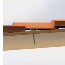
4. Screw the 5/16" lag bolt into rafter, embedded a min. of 2.5" (*Tightening torque depends on the planned location.)
