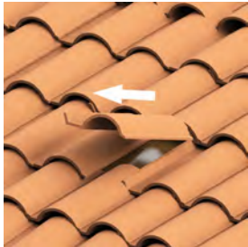
1. Remove the tile and locate the rafter.
