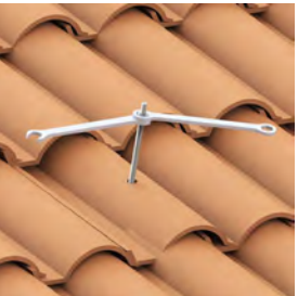
7. Use two wrenches to attach the 3/8" nut to the threaded headless bolt. Attach to the channel nut below the tile and remove the nut when done.
