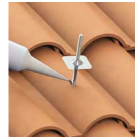
8. Apply fresh compatible sealant to seal the tile opening and lower the mini flashing.
